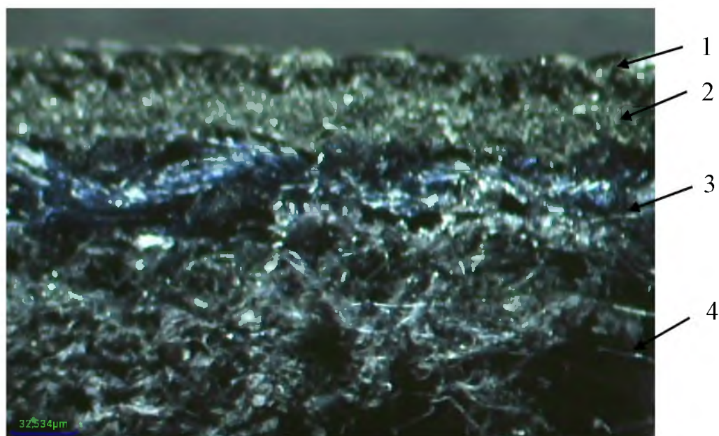
1- finishing layer, 2 – nanopur layer, 3 – woven fabric, 4 – leather layer Figure – Microscopic image of Eco-leather
